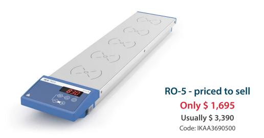
5-position digital magnetic stirrer without heating, designed for synchronous stirring. The magnetic coil technology provides noiseless and consistent stirring on all positions. Speed remains constant, even when load changes.
